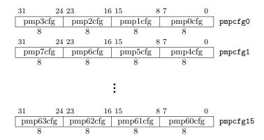
Figure 3.31: RV32 PMP configuration CSR layout.
