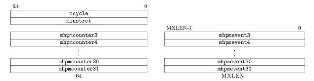
Figure 3.16: Hardware performance monitor counters.
