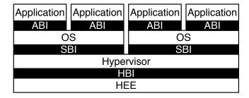
Figure 1.1: Different implementation stacks supporting various forms of privileged execution.
