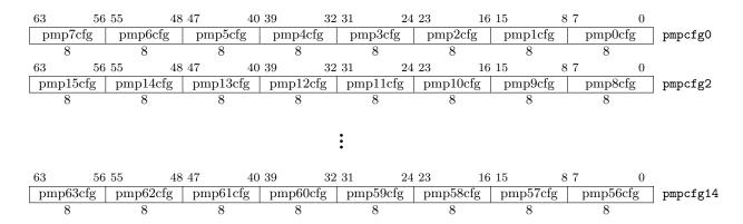
Figure 3.32: RV64 PMP configuration CSR layout.
